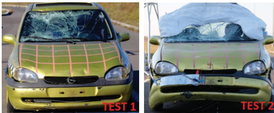
Fig. 2. Cyclist head impact location for each crash-test
