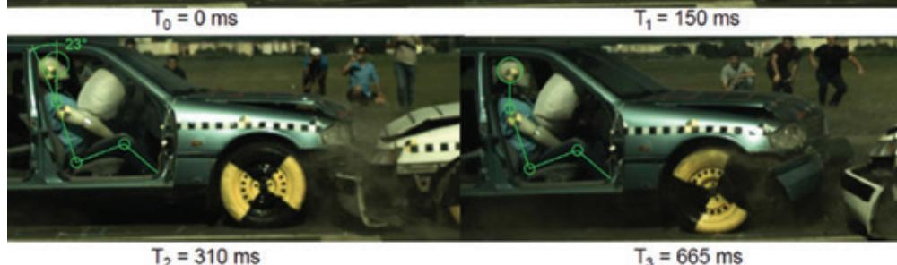
Fig. 12. Kinematic analysis of the occupant during the second test
