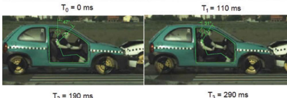
Fig. 11. Kinematic analysis of the occupant during the first test
