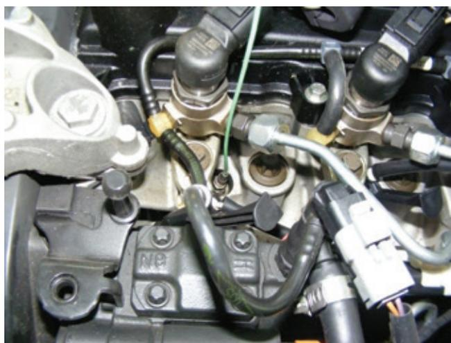
Fig. 2. In-cylinder pressure sensor
